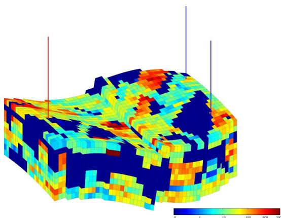
Fig. 3. Permeability distribution, where red indicates high permeability zones while blue shows low permeability zones, of the reservoir model. The red line indicates the production well location, the blue line on the right corresponds to injector well 1 and the blue line on the left corresponds to injector well 2.
