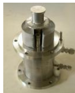
Fig. 4. Jet Co-flow Packing Trays (JCPT) with Catalyst Package.
