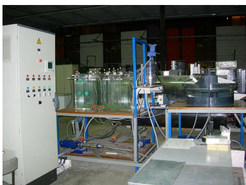
Fig. 1. The activated sludge pilot plant
