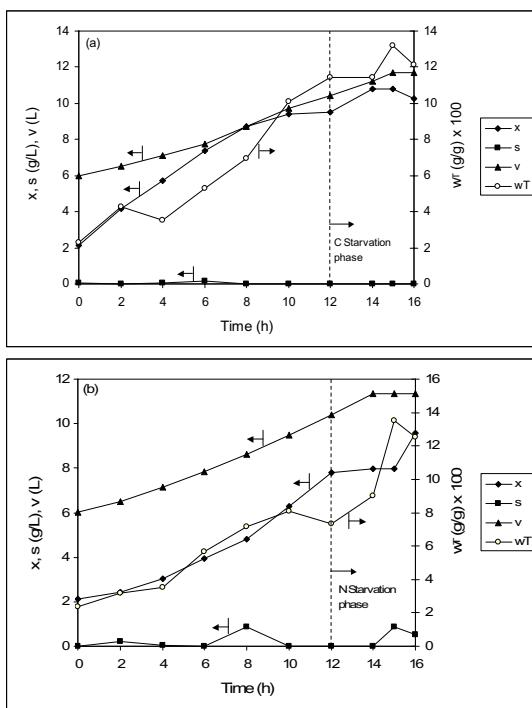
Figure 1. Biomass ( $x$ ), substrate ( $s$ ), intracellular trehalose ( $w_T$ ) and culture medium volume ( $v$ ) as functions of time during a yeast production process depleted in (a) carbon source and (b) nitrogen source, in the last three hours of the process.
