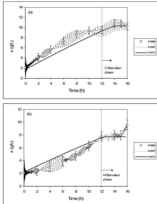
Figure 3. Estimation of biomass concentration in a yeast production process. Empty marks represent experimental values, dotted line is the DNNO estimations and solide line gives the numerical values of the structured model for (a) carbon-starved and (b) nitrogen-starved yeast cultures.
