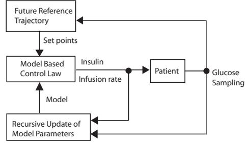
Fig. 1. Block diagram of the control strategy
