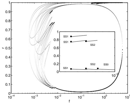
Fig. 2. Bifurcation diagram of  $r$  vs  $f$  for a 4-CSTR bidirectional network with  $k = 25$ ,  $d = 0.1$ , and  $g = 0.002$ . Unstable steady states are indicated with a light line and stable steady states are indicated with a dark line. Inset: stable steady state detail. The  $\blacksquare$  symbol represents a Hopf bifurcation point.
