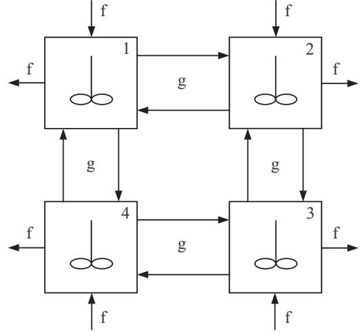
Fig. 1. 4-CSTR network schematic
