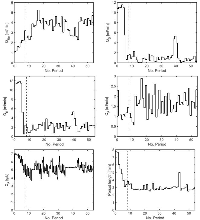
Fig. 3. Optimal dynamic experiment for the estimation of isotherm parameters of the individual columns of the SMB plant. The inputs starting from the 8th period are calculated with online experiments.
