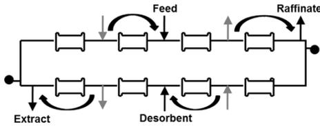
Fig. 2. Schematic representation of the SMB process.
