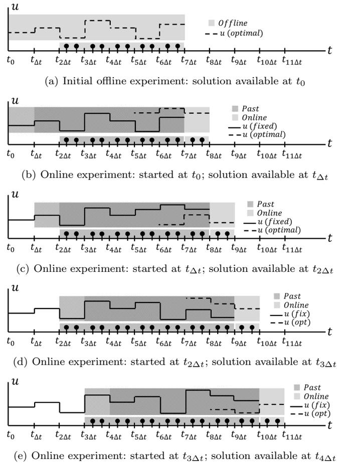
Fig. 1. Schematic representation of the online experiment design method for four consecutive  $\Delta t$  segments.
