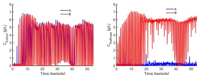
Fig. 4. Concentrations measured at the extract (left) and raffinate (right) ports.
