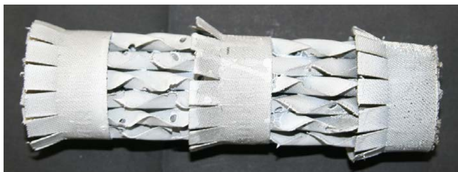
Figure 4: Sol-gel coated wire gauze packing Sulzer BX
