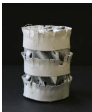
Figure 1 - Silica-based coating for immobilization of lipase CALB on structured packing (Montz A3-500 or Sulzer BX)
