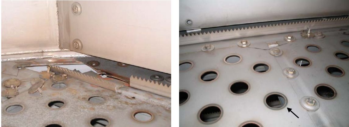
Figure 3: Typical failure patterns of V1-valve trays
