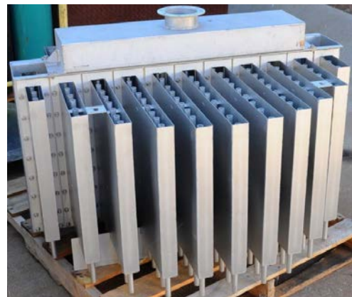
Figure 2 High turndown narrow trough Type-R Montz liquid distributor. (Courtesy of Dr. S. Chambers of FRI).
