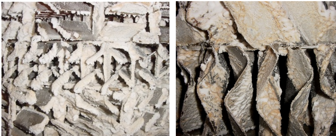
Figure 3: Accelerated fouling tests on conventional grid packing (left) and PROFLUX™ severe service grid (right)
