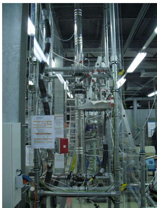
Figure 5: Experimental setup for the reactive distillation investigation (a), configuration of the RD column (b).
