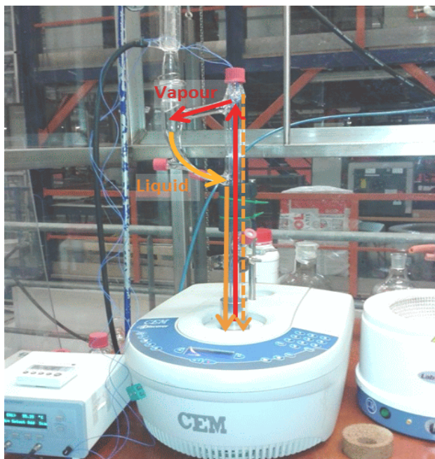
Figure 1: Lab scale distillation setup for microwave experiments, flowing conditions indicated.
