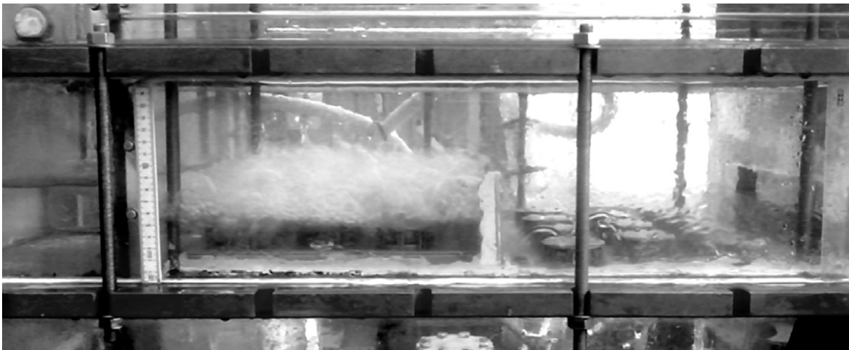
Figure 7: Water/air tests at nominal load exhibiting VPC.
