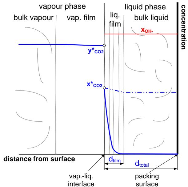
**Figure 5.** Two-film model acc. to Whitman CO<sub>2</sub> concentration profile with and without reaction.
