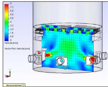
Fig. 3: CFD analysis of gas inlet
