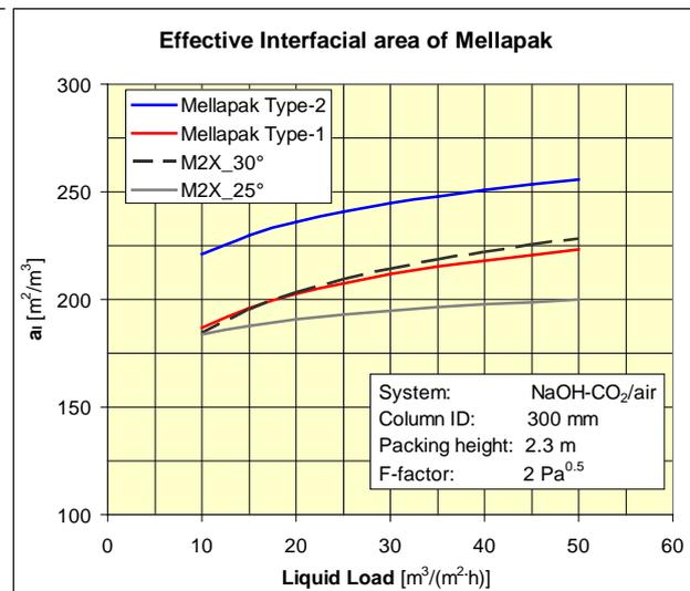
**Fig. 7:** Efficiency of new Mellapak Type-1 and Type-2 compared to M2X
