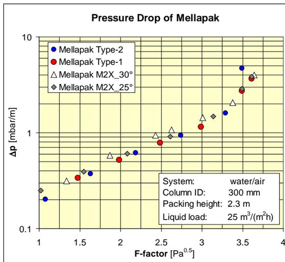
**Fig. 6:** Pressure drop of new Mellapak Type-1 and Type-2 compared to M2X
