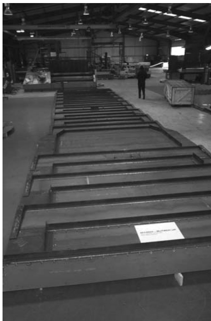
Figure 6. Trial assembly of DW at Koch-Glitsch
