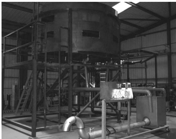
Figure 4. Liquid splitter test rig at Koch-Glitsch
