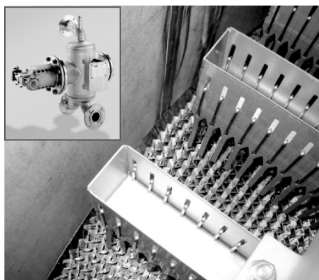
Figure 6. Photographs of the details of the liquid distribution system for very low loads
