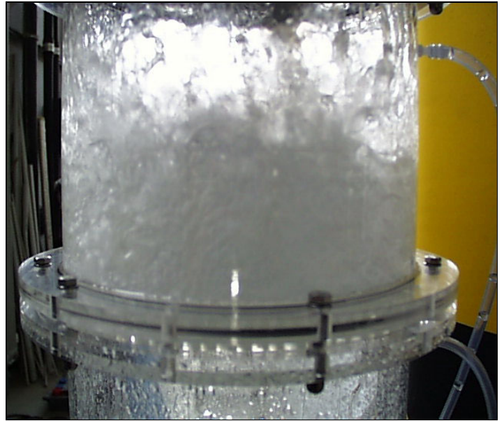
Fig.9: View of the Tray During Operation
