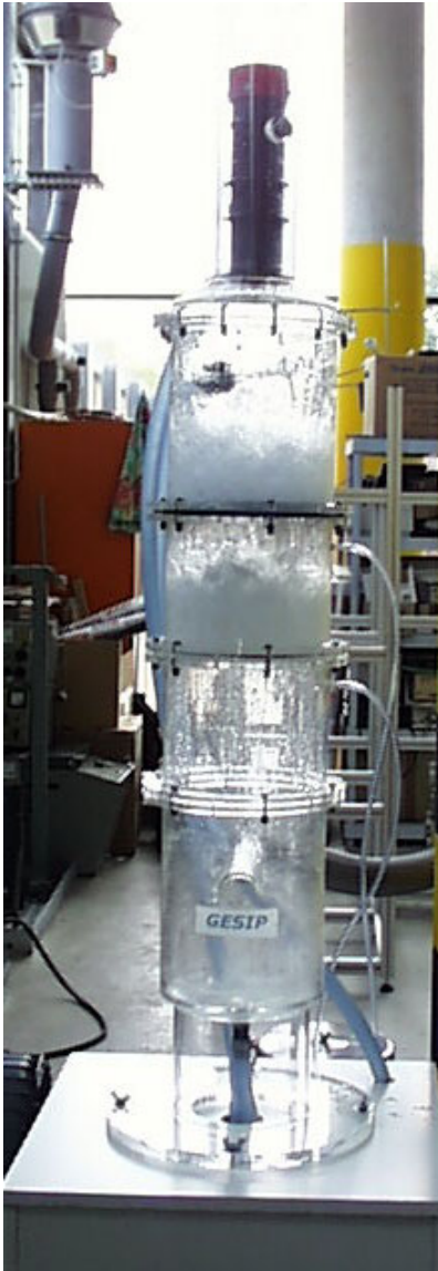
Fig.13: Test column with sieve tray with froth stabilizer
