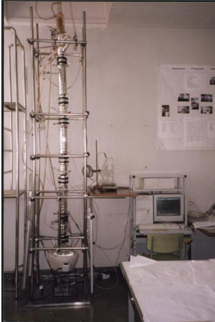
*Figure 2. Batch distillation pilot plant.*
