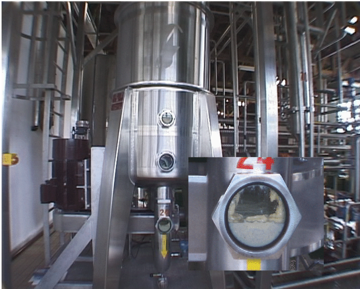
Figure 2: A Flavourtech Model 10,000 SCC being used to process banana puree. Inset is an enlarged view of the sight glass in the discharge line, showing the puree being pumped out of the column. The flow rate was 3,500 L/h.
