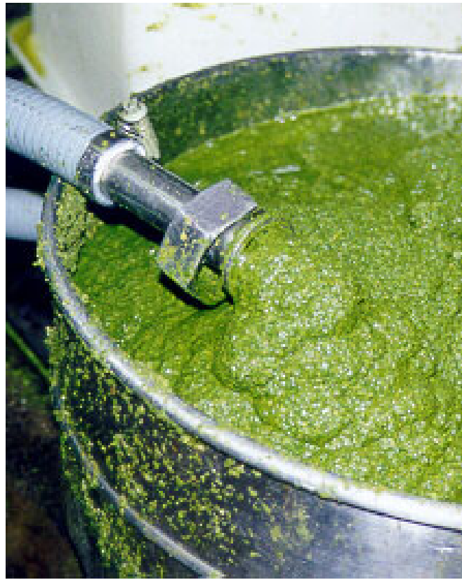
Figure 1: A 10% slurry of green tea being discharged from a Model 500 SCC after stripping of volatiles. The flow rate was 300 L/h.
