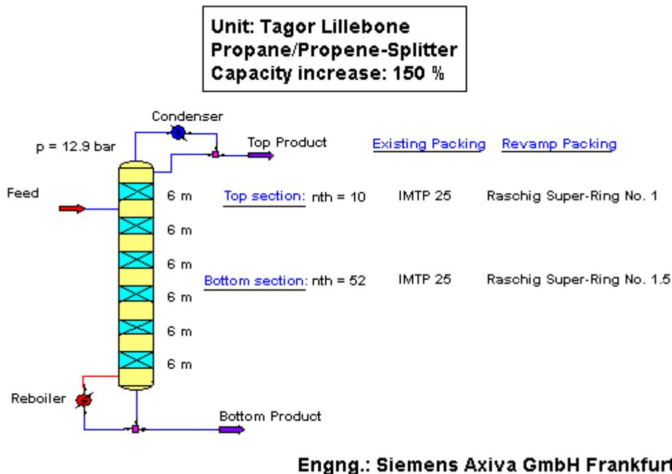
*Fig. 16: Revamp of a C<sub>3</sub>-Splitter from IMTP 25 to Raschig Super-Ring No. 1 and No. 1.5*
