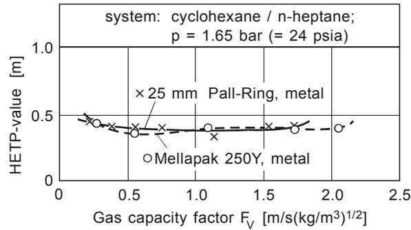
Fig. 7: HETP-value for 25 mm Pall-Ring and Mellapak 250Y for rectification system cyclohexane/n-heptane at 1.65 bar. Tests had been performed at FRI facility in Stillwater Oklahoma/USA.
