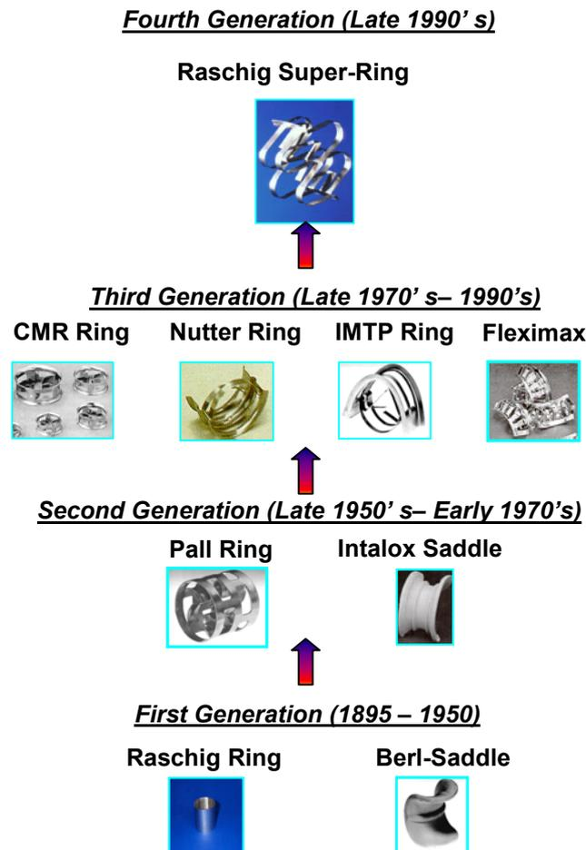
*Fig. 1: History of development of characteristic random packings of different generations*
