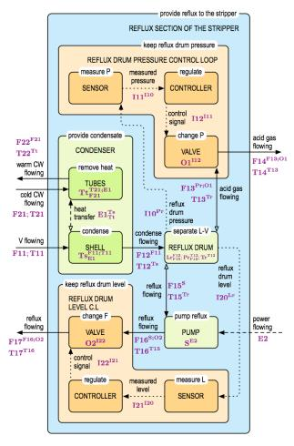
Figure 5. D-higraph of the reflux section of the stripping part of the amine process.
