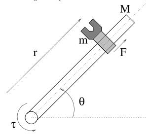
The arm is modeled as a segment with mass M and length L, and the hand as a point with mass m. Denoting by r the position and by  $\theta$  the angle of the arm, the resulting equations are:
