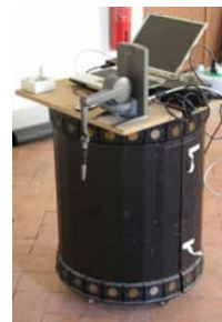
Fig. 1. A general purpose interface based on the holonomic Nomad mobile robot and a Phantom
