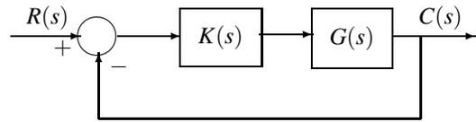
Fig. 1. Closed-loop feedback control system
