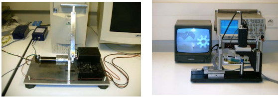
Fig.10: Master-slave experimental micromanipulation setup.
