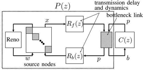
Fig. 2: The closed loop controlled system for one bottleneck link congestion
