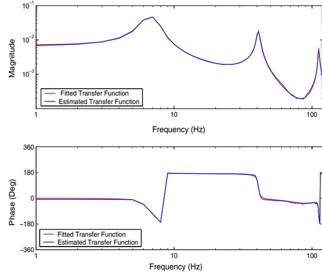
Fig. 2, Frequency response of the flexible beam.
