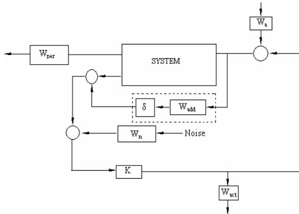
Fig.3, Block diagram of the  $H_\infty$  Controller
