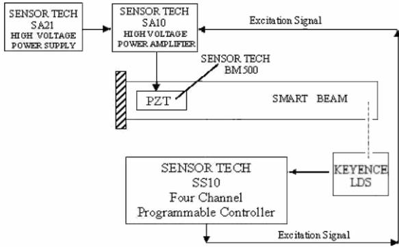
Fig.5, Experimental setup of the flexible beam system
