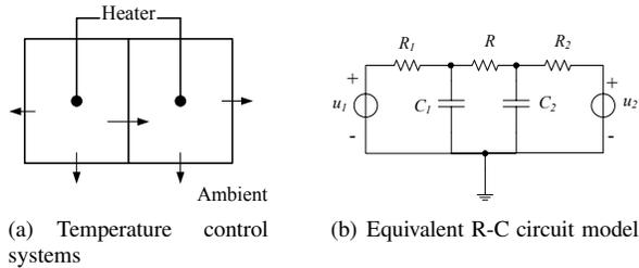
Fig. 2. Dynamics of a two-room temperature control system.
