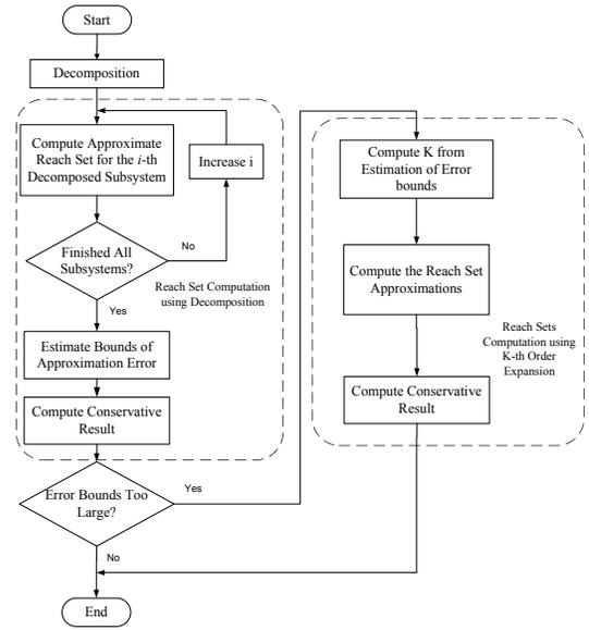
Fig. 1. Computation procedure.
