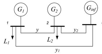
Fig. 4. A three-bus power system.
