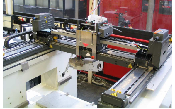
Fig. 2. The adapted H-bridge setup.
