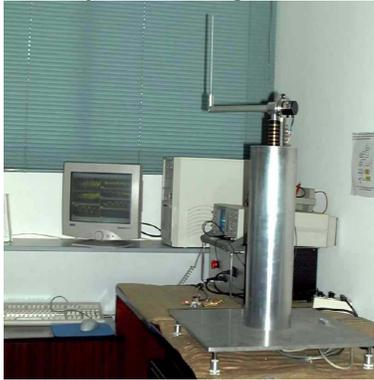
Fig. 3. Experimental rotary pendulum system.
