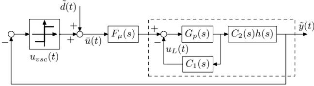
Fig. 6. Equivalent control scheme of *Theorem 5*.
