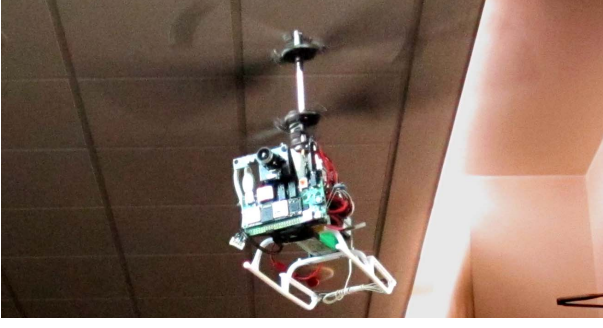
Fig. 1: The instrumented miniature co-axial helicopter in actions. The model is of EK1H-E020 from E-sky.
