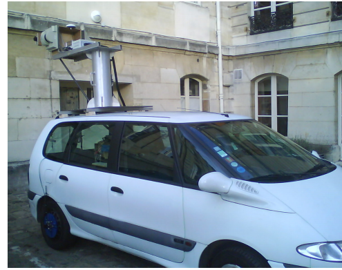
Fig. 3. Used vehicle and IMU/GPS on the roof
