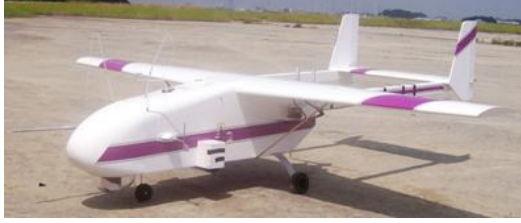
Fig. 3. Fixed-wing UAV used in the camera-in-the-loop simulation
