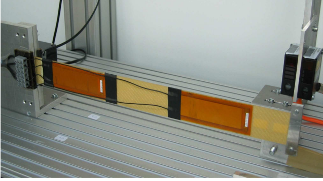
Fig. 2. Picture of the cantilevered beam with two pairs of MFC actuators and tip mass.
