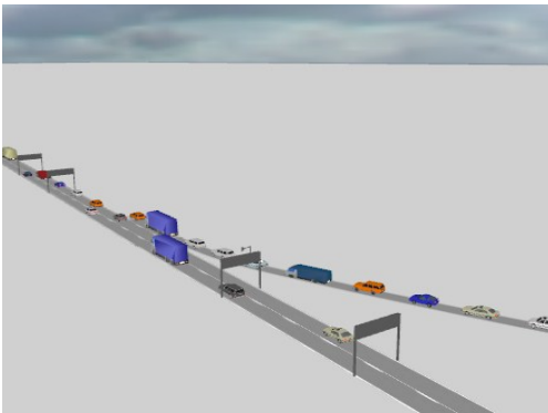
Fig. 1. Instant of 3D freeway traffic simulation with ITS signals (ramp metering and variable speed limits) using Aimsun 6.0
