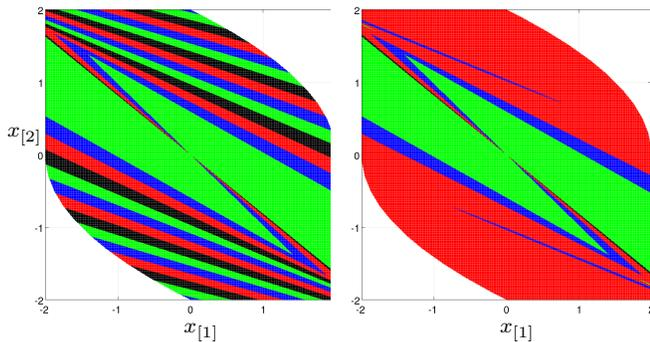
Fig. 6. Constrained asynchronous case: State-dependent optimal initial inter-period step:  $j^*(x) = \{0, 1, 2, 3\} = \{\text{black}, \text{red}, \text{blue}, \text{green}\}$ . Optimal (left), sub-optimal (right).
