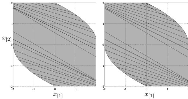
Fig. 4. Asynchronous constrained case: Optimal (left, number of regions:  $\sigma_1 = 21$ ) and sub-optimal (right, number of regions:  $\sigma_1 = 31$ ) PWQ running cost function partition.
