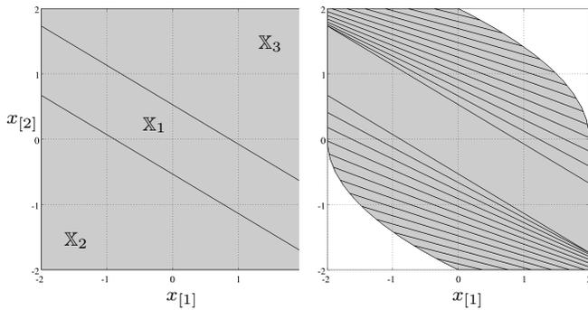
Fig. 2. Synchronous constrained case: PWA optimal LQR control law partition (left), and resulting PWQ running cost function partition (right). Number of regions in PWQ partition:  $\sigma_1 = 27$ .
