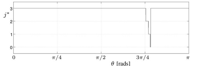
Fig. 5. Unconstrained asynchronous case: State-dependent optimal initial inter-period step  $j^*(x)$ ,  $x = [\cos(\theta) \sin(\theta)]^T$ .
