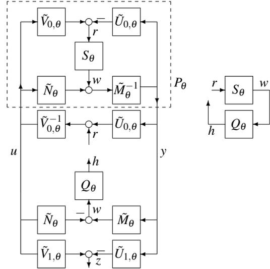
Fig. 2. Left: Plant-controller interconnection represented by dual Youla and Youla parametrisations. Right: Corresponding internal loop.
