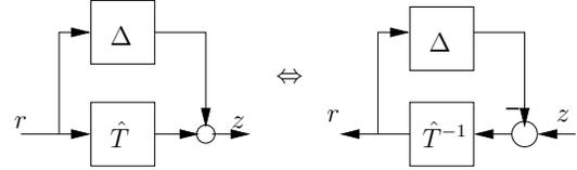
Fig. 3. Inversion of  $T$  as a feedback loop.
