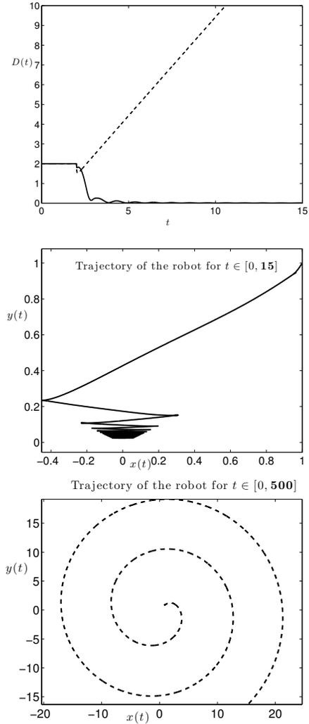
Fig. 2. The delay and the trajectory of the robot with the delay-compensating controller (top two plots) and the trajectory of the robot with the un-compensating controller (bottom plot).
