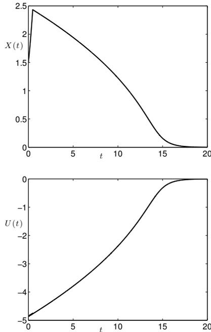
Fig. 4. Response of system (49) with the predictor controller and initial conditions as  $X(0) = 1.5$  and  $U(\theta) = 0$  for all  $-\frac{1}{4} \log(X(0)^2 + 1) \leq \theta \leq 0$ .
