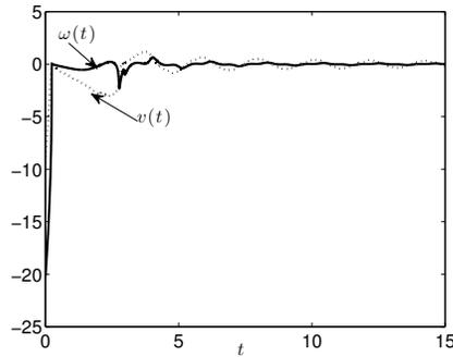
Fig. 3. The control efforts  $v(t)$  (dot line) and  $\omega(t)$  (solid line) for the non-holonomic unicycle with the delay-compensating controller.
