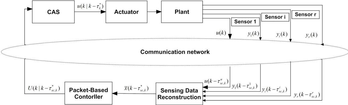
Fig. 2. Model-based compensation for NCSs with multi-packet transmission.
