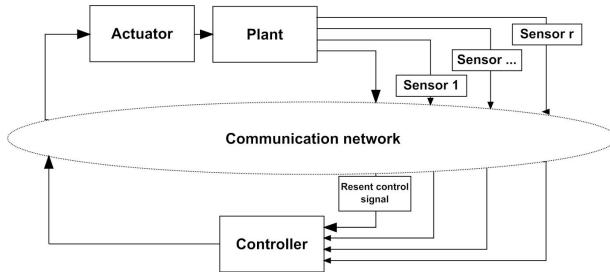
Fig. 1. Multi-packet transmission due to geographically dispersed sensors.
