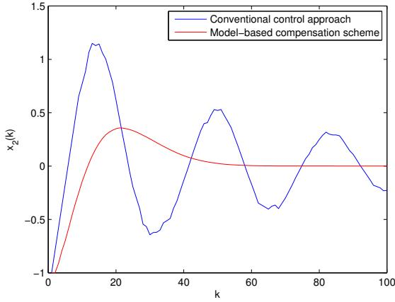
Fig. 3. State trajectories using the LQR controller and the model-based compensation scheme, respectively. Showing only the second state.
