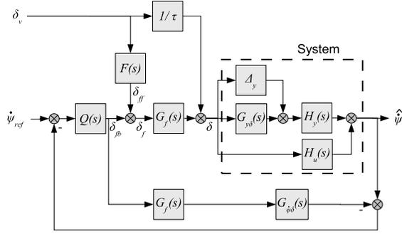
Fig. 2. Control structure using a virtual sensor.
