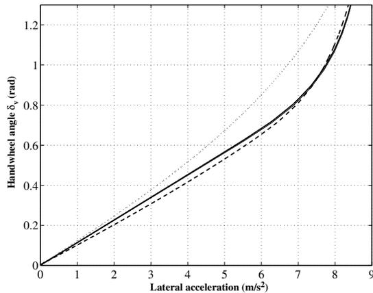
Fig. 3. Steering pad test at 100 km/h. Thin line: reference steering diagram. Comparison between the steering diagrams obtained with the uncontrolled vehicle (dotted) and with the controlled ones using either yaw rate sensor (solid) or DVS (dashed).
