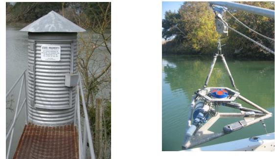
Fig. 7. Left: USGS Sensor station at GSS, used as a measurement sensor. Right: Deployable ADCP sensor, used in Section 3.5 for gathering the validation data (three of them were deployed between 11/01/2007 and 11/12/2007 in order to gather the data for this study).
