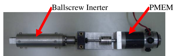
Figure 1. The prototype of a mechatronic suspension strut.
