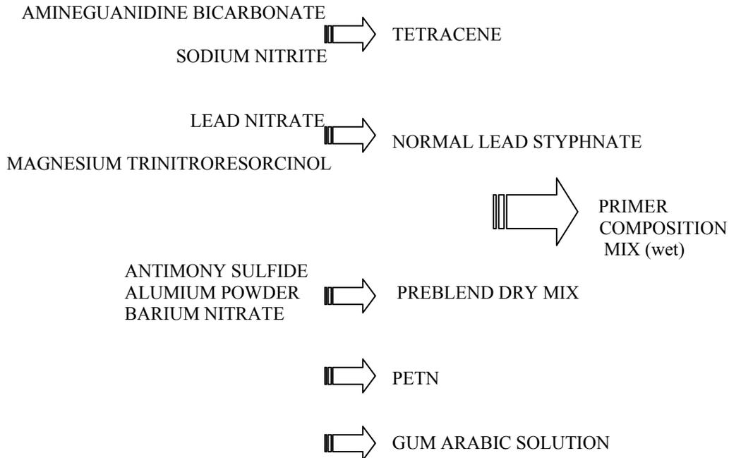
The wet-mixing procedure consists of the following steps:
