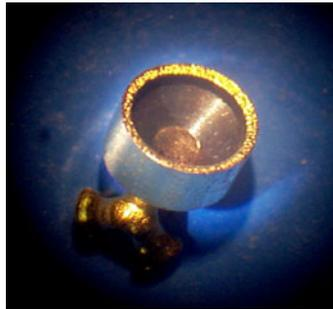
**Figure 1 – No. 41 Small Caliber Percussion Primer Showing Loaded Cup and Tripod Anvil**
