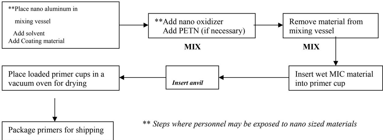
**Figure 4 - Proposed MIC Primer Manufacturing Process**
