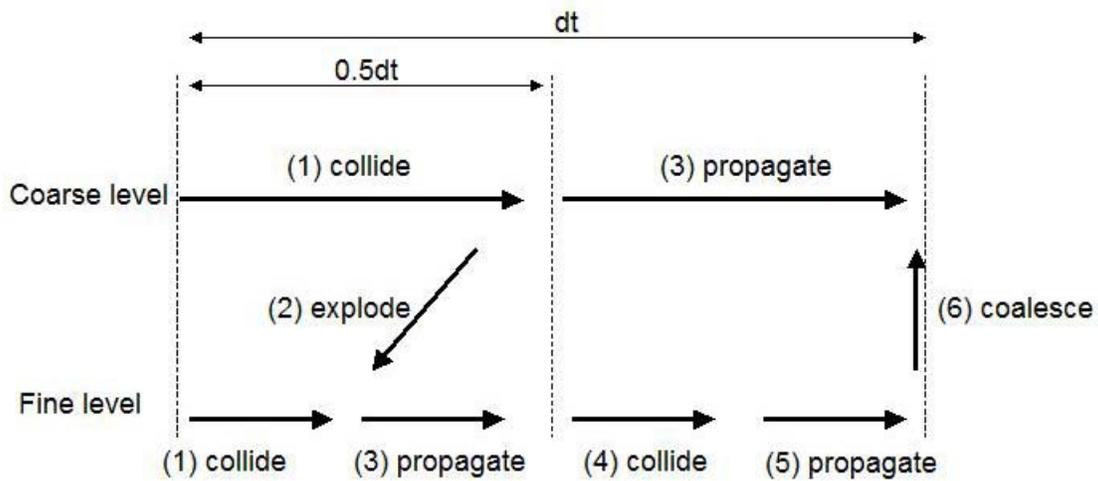
Figure 2. Flowchart of the computation steps for two refinement levels
