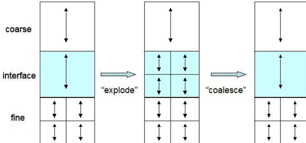
Figure 1. Schematic plot showing the “explode” and “coalesce” operation at refinement jump
