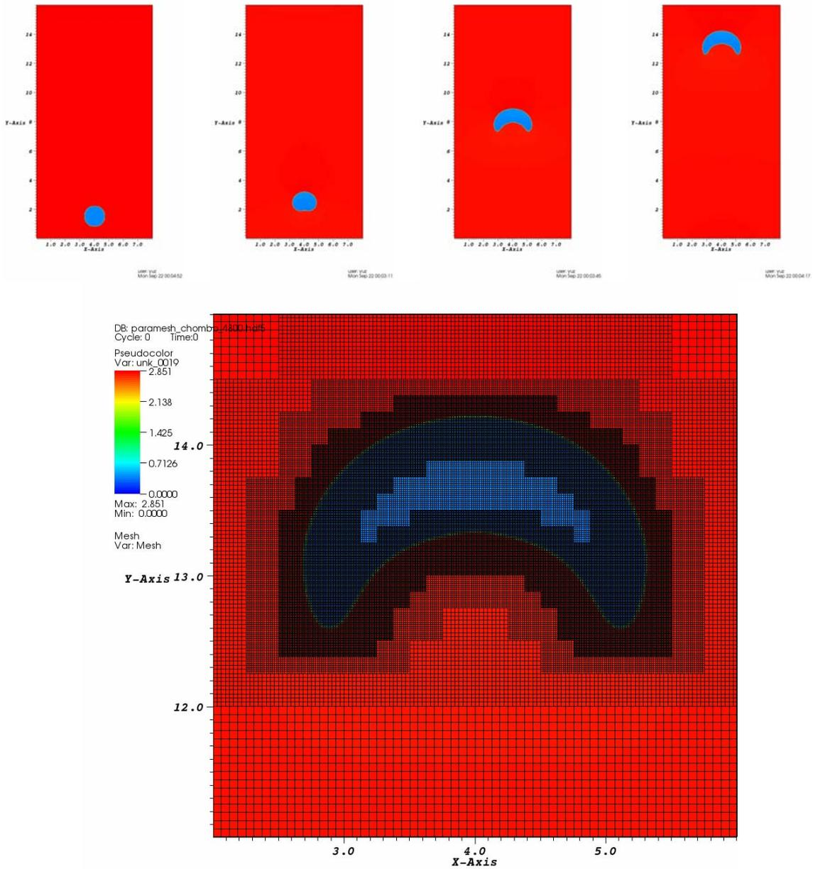
Figure 5. Ellipsoidal cap bubble.  $Eo=62$ ,  $Mo=135$ .
