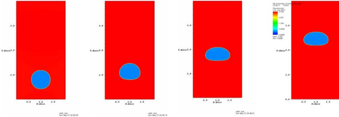
Figure 4. Ellipsoidal bubble.  $Eo=4.1$ ,  $Mo=3.3 \times 10^{-4}$ .
