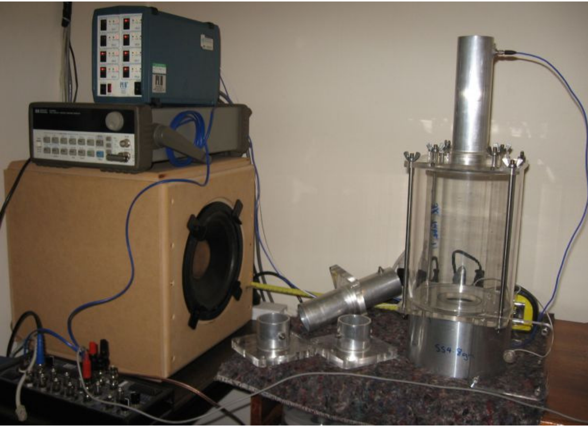
Figure 11. Photograph showing experimental equipment: loudspeaker, left; resonator, right; signal generator on top of loud speaker.
