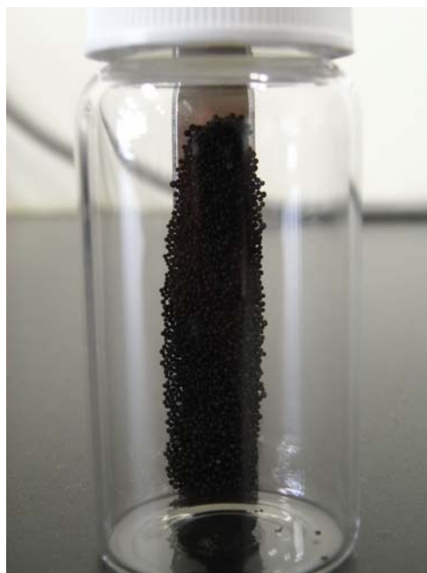
Figure 1: Photographs of prepared Co/IR-120 catalysts placed in bottle in a magnetic field with magnetic strength near 12,000 G show their intrinsic magnetism.
