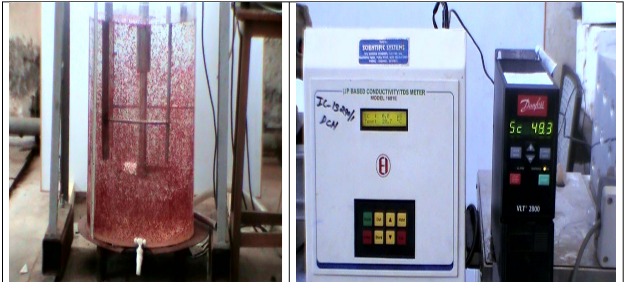
1.Flat Bottom Tank, 2.Baffles, 3. A 4 junction Thermopile, 4.Hydrofoil Agitator, 5. Motor Shaft, 6. Water Bath, 7. Motor Controller drive, 8. Digital Multimeter, 9. 3P Electric Motor, 10. Temp. Controller, 11. Humidity Meter, 12. Inlet port
