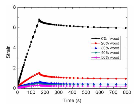
Figure 4. Strain Response of HDPE-Wood Composites.
