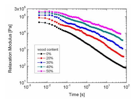
Figure 5. Relaxation Modulus of HDPE-Wood Composites.
