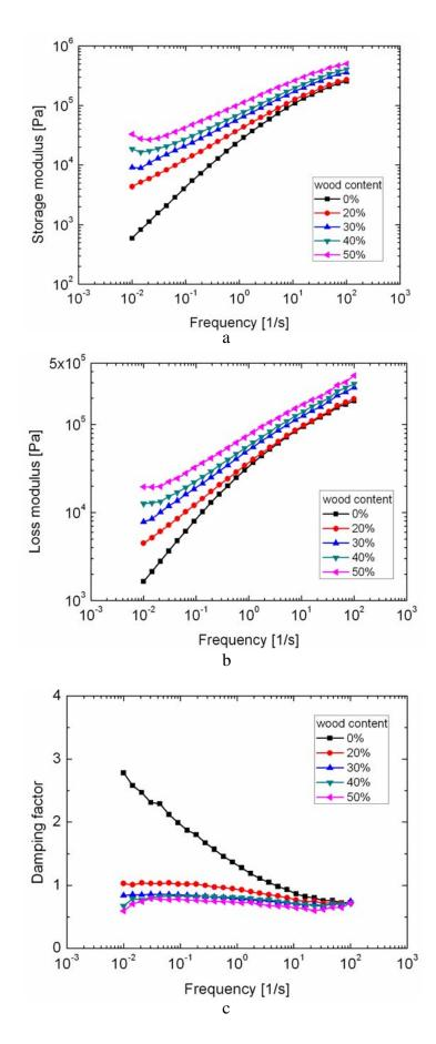
**Figure 2.** Storage Modulus (a), Loss Modulus (b) and Damping Factor (c) of HDPE-Wood Composites.
