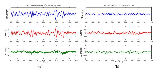
Figure 10: Time series where the demand forecast is developed from (a) an OE-[1 2 1] fit to unfiltered data  $(\Sigma(y-r)^2 = 203, \Sigma(\Delta u)^2 = 5)$  and (b) an OE-[1 2 1] fit to control-relevant filtered data  $(\Sigma(y-r)^2 = 14, \Sigma(\Delta u)^2 = 2)$  obtained from the user defined weighting function ( $\gamma = 0.3$ ).
