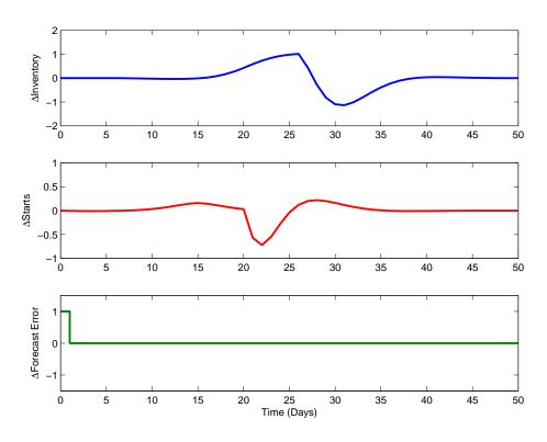
Figure 4: Supply chain control system response to a unit forecast error pulse. Throughput time:  $\theta = 5$  days, prediction horizon: p and  $\theta_F = 20$  days, move horizon: m = 10 days, move suppression:  $Q_{\Delta u} = 5$ , control error weight:  $Q_e = 1$ .
