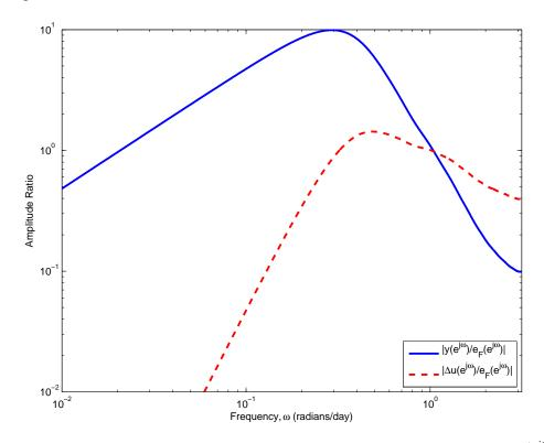
Figure 5: Amplitude ratio of the inventory and starts change response to forecast error  $\left(\frac{y(e^{j\omega})}{e_F(e^{j\omega})}\right)$  and  $\frac{\Delta u(e^{j\omega})}{e_F(e^{j\omega})}$ , respectively) for the model and controller parameters per Fig. 4.
