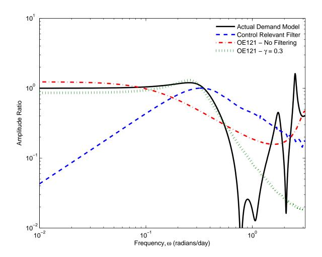
Figure 9: Corresponding frequency responses where the demand forecast is developed from an OE-[1 2 1] fit to unfiltered data and an OE-[1 2 1] fit to control-relevant filtered data obtained from the user defined weighting function ( $\gamma = 0.3$ ).
