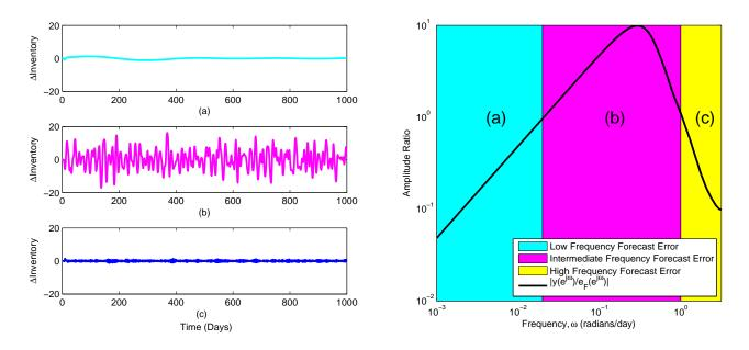
Figure 6: Inventory response of the closed-loop production/inventory system to low frequency (a), intermediate frequency (b), and high frequency forecast error (c).
