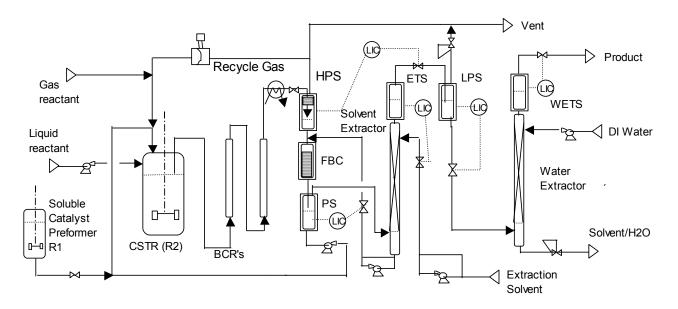
Figure 1: New Pilot Concept with Re-Use of Reaction Section
