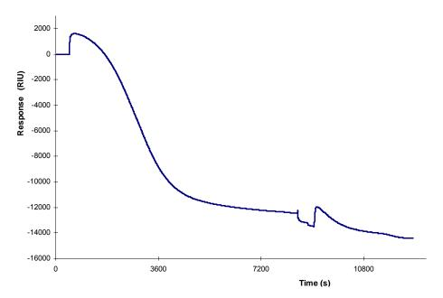
Figure 2. Change in Refractive Index Units (RIU) as the response of a SPR to endoglucanase binding and cellulose degradation
