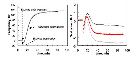
Figure 1. Change in frequency (left) and dissipation (right) by enzyme. The different lines represent the different overtones (or harmonics): f3/3 (black line), f5/5 (red) and f7/7 (light grey). The driving frequencies correspond to 15, 25 and 35 MHz for f3, f5 and f7, respectively.
