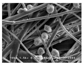
Figure 4. Scanning electron micrograph of KG-1a cells adhering to PNIPAAm-g-PP membrane that had been soaked in anti-human CD34 mAb (10  $\mu$ g/mL PBS) at 37 °C for 2 h. Scale bar = 6.67  $\mu$ m.
