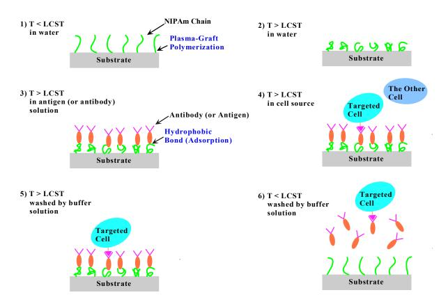
Figure 1. Schematic mechanism of cell separation using PNIPAAm-g-PP membrane.
