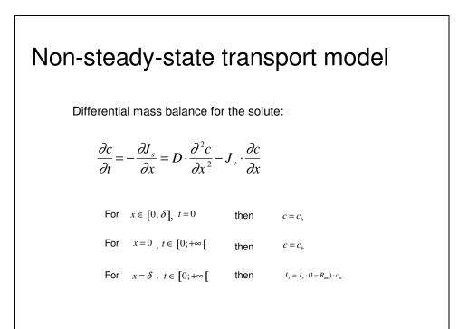
The differential equation is solved as a difference equation in a work sheet assuming a constant boundary layer thickness and a constant retention of the membrane,  $R_{int}$ , in which case the permeate concentration is related to the concentration at the membrane surface as shown in Fig. 3. Further the average permeate concentration and average permeate flux are calculated by a summation from time zero to the actual time before an eventual backflux is started.
