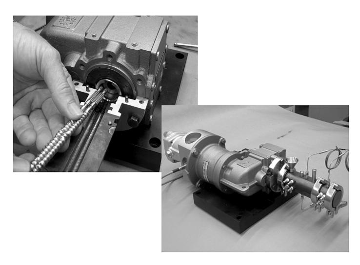
Mini extruder specifically designed for processing of nanoenergetics
